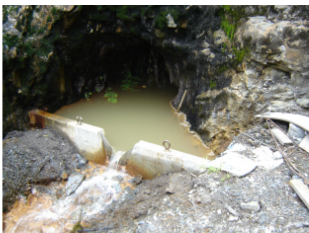
Plate 5: V-notch weir at adit outflow.
