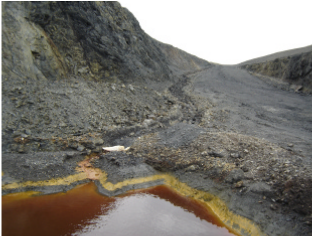
Plate 3: Sediment trap and drain in Allion's decline.
